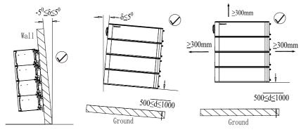
Fig 4.1:Acceptable wall mounted installation
