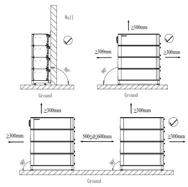
Fig 4.2:Acceptable floor standing installation
