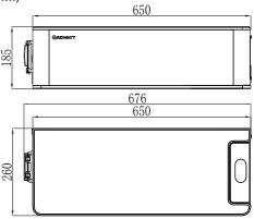
Fig 1.2: Dimension of HVC 60050-A1
