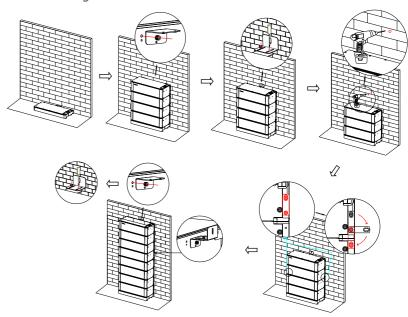
Fig 4.8: Floor standing installation process
