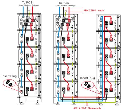
Fig 4.9: Single line installation
